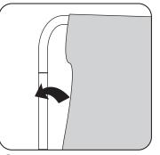
Once the fabric is on the frame, zip the fabric over the vertical pole.
