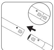
1 Assemble the frame by clicking together the poles. Use the stickers found on the end of each pole piece to identify the proper corresponding connections.
