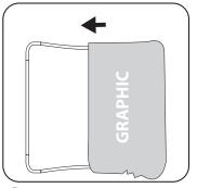
Pull the fabric over the side frame and pull the top and bottom evenly. The fabric may catch a bit on the tube joints, just pull the fabric out and over to continue.
