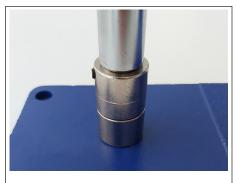
6. Periodically pull down on the handle (A) to ensure the bottom die (D) is perfectly in line with the top die (C). Repeat step 5 until the top and bottom are perfectly aligned.
