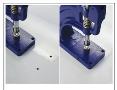
To fasten the Max-Press to a work surface, use the 4pcs socket cap screw and nuts (G) in each of the four corners of the main body (B).
