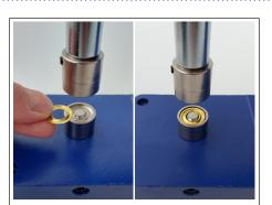
**2.** Place the bottom part of the grommet into the Bottom Die (D).
