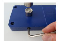
**4.** Secure the bottom die (D) into place. Slowly tighten the screws in the base of the main body (B) with the hex key (E).
