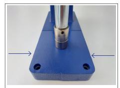
**5.** Adjust the bottom die (D) by loosening/tightening the two screws on either side of the base to re-position the bottom die (D) left or right, while adjusting it forwards and backwards as required.
