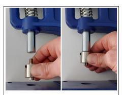
**2.** Thread the top die (C) into the main body (B). Tighten by hand only; **do not** use tools.
