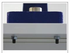
Thread the nuts onto the end of the four socket cap screws (G) under the work surface to secure the Max-Press in place.
