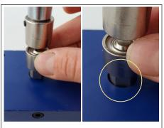
**3.** Place the bottom die (D) into the base (B). Ensure the flat sides of the bottom die (D) are facing towards the sides of the main body (B).
