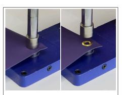
**3.** Insert media (print side up). Pull down on the handle (A) applying necessary pressure and voilà!
