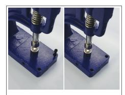
2. The heads of the socket cap screws (G) should sit in the holes of the main body (B) so that they are flush with the surface of the base.
