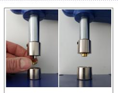
**1.** Push the top part of the grommet up onto the Top Die (C).
