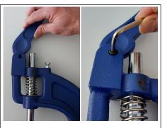
**1.** Attach the handle (A) to the main body (B) with the hex key (E) and socket cap screw (F).
