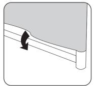
Once the fabric is on the frame, it is easiest to lay the frame down to zip the fabric under the bottom horizontal pole.
