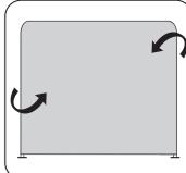
These frames can easily be adjusted if there is a twist to the frame after the fabric is on. Simply twist the frame until it is flat. The tension of the fabric will hold it where you set it.
