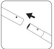
Assemble the frame – less the feet – by clicking together the poles.
