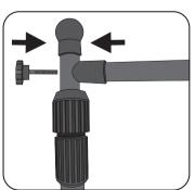
Attach the horizontal poles to the vertical support poles using the large screws found in the end of each horizontal pole. Adjust the direction of the feet
