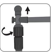
Adjust the graphic height by rotating the pole extension locks to loosen the telescopic pole. Pull to the desired length, and gently tighten the pole extension locks. DO NOT overtighten to eliminate the small gap.
