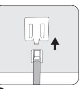
6 Slide the top clips on the header poles into the channels found on the back of the header.
