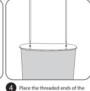
Place the threaded ends of the header channel poles through the holes found on the countertop.
