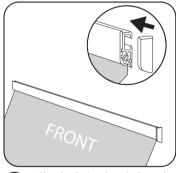
Place the plastic end caps back onto the bottom bar.
