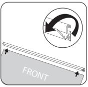
Open the bottom bar and fully insert the bottom of the banner (front facing up).
