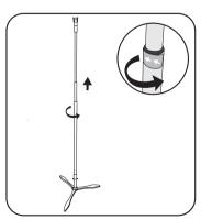
Open the support feet, and place the base onto the ground. Gently twist the support pole to extend to desired height, and gently twist to lock pole in place. DO NOT OVER LOOSEN OR OVERTIGHTEN THE SUPPORT POLE.
