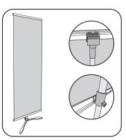
Attach the bottom bar to the bottom clip, then attach top bar to top clip on the support pole. Repeat for additional graphic.
