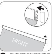
Place the plastic end caps back onto the top bar.
