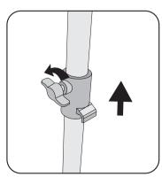
Rotate knob on bottom clip and place at desired height. DO NOT OVERTIGHTEN KNOB.
