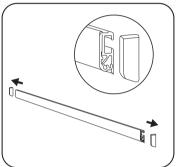
Remove the plastic end caps from the clamp bottom bar.
