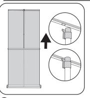
Tilt the top bar back on a slight angle to position the fitting at the top of the pole into the channel in the center of the top bar. Repeat steps 2 to 3 for additional graphic
