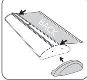
Repeat steps 7 to 10 for additional graphic. Store both locking pins in the end cap and place the end cap back onto the base
