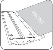
Peel the paper off the adhesive along the edge of the leader. Ensure the bottom of the banner is straight along the adhesive, and attach the banner (front facing up).
