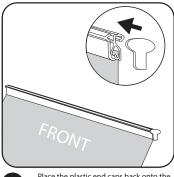
Place the plastic end caps back onto the top bar (repeat steps 2 to 5 for additional graphic).
