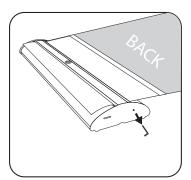
Gripping the banner securely with one hand, remove the locking pin, closest to the side you are planning to retract, from the side of the base.
