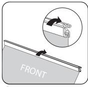
Press down firmly on clamp top bar to secure graphic into place.
