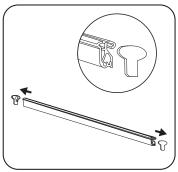
Remove the plastic end caps from the clamp top bar.
