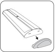
Remove the end cap to expose the locking pins.
