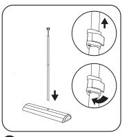
Assemble pole and insert the bottom of the pole in the center of the base. If the pole is telescopic, raise pole by opening latch, and secure at desired height.
