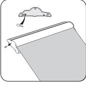
Gripping the banner securely with one hand, remove the locking pin from the left side of the base. Store the locking pin in the chrome end cap.
