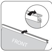
Press down firmly on clamp top bar to 4 secure graphic into place.
