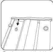
Remove the screw holding the left end cap, and remove it.
