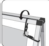
Loop the bungee hooks through the grommets and over the horizontal poles and vertical support poles on the A-frame at each corner. Then loop the bungee hooks through the grommets andover the horizontal poles near the center A-frames to finish securing the banner. Repeat for additional graphic.
