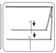
6 Secure to soft ground by placing ground stakes over bottom horizontal poles.
