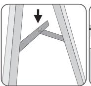
Once the unit is assembled, stand it upright and extend the four A-frame hinges until it stands on its own.
