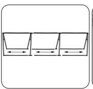
Place the two end A-Frames so they are spaced approximately 12ft apart with the black connectors facing each other, and the center A-frame in the middle. Place the horizontal poles between the top and bottom connectors on both of the end A-frames and the center A-frames.
