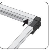
Connect the horizontal poles with the A-frames by inserting the black connecting joints into the open ends of the poles.
