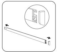
Remove the plastic end caps from the clamp top bar.
