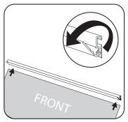
Open the clamp top bar and fully insert the top of the banner (front facing up).
