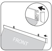
Place the plastic end caps back onto the clamp top bar.
