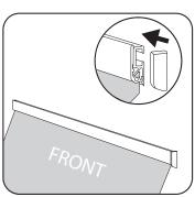
Place the plastic end caps back onto the clamp bottom bar.
