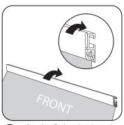
Press down firmly on clamp bottom bar to secure graphic into place.
