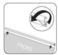
Open the clamp bottom bar and fully insert the bottom of the banner (front facing up).
