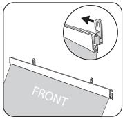
Slide the hanging clips onto the top bar inside the channel found on the back of the clamp top bar.
