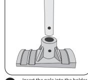
Insert the pole into the holder on the bracket. Line the hole on the end of the pole with the holes on the side of the pole channel on the bracket.
