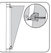
To mount graphic to a D-bracket, thread zip tie through loop in D-bracket and through the grommet on the bottom of the banner.
