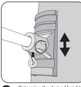
Determine the desired height of the streetpole. Position the top bracket with the tapered end pointing up.
