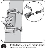
Install hose clamps around the street pole and bracket. Tighten clamp with a 5/16" hex head wrench/nut driver.
