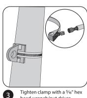
Tighten clamp with a 5/16" hex head wrench/nut driver.
