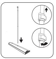
Assemble pole and insert the bottom of the pole in the center of the base. Ensure the pole is fully inserted onto the plastic fitting at the bottom of the base. Raise telescopic pole by opening latch, and secure at desired height.
