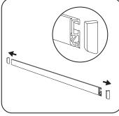
Remove the plastic end caps from the clamp top bar.
