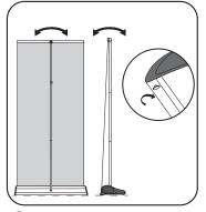
Adjust the threaded feet concealed underneath the base to level the unit if required.
