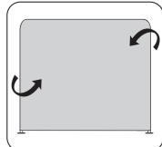
These frames can easily be adjusted if there is a twist to the frame after the fabric is on. Simply twist the frame until it is flat. The tension of the fabric will hold it where you set it.
