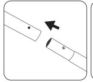
Assemble the frame – less the feet – by clicking together the poles.
