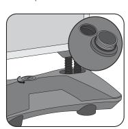
6 Ballast can be added to base by removing the twist-off cap at the center of the base. Antifreeze additives or sand are recommended for use below 0°C (32°F).
