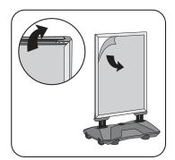
4 Open all four edges of the snap frame. Remove the protective graphic cover (P).
