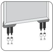
Remove nuts (D) that arrive secured to the bolts (beneath springs) and set aside for later use. Discard the four protective foam tubes.
