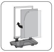
5 Slide the graphic into the frame, followed by the protective graphic cover (P). Snap the profile closed. \*Repeat on both sides.
