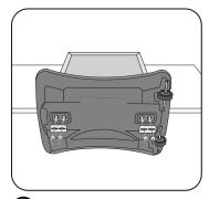
Resting the unit on its side, place a metal plate (C) over the protruding bolts and secure with two nuts (D). Tighten using included wrench. \*Repeat on both sides.
