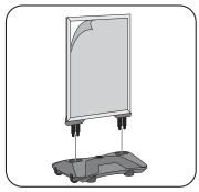
2 Insert the spring legs on the snap frame (A) through the holes on the top of the fillable base (B).
