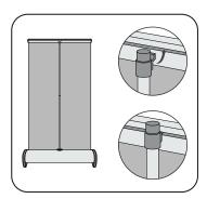
Tilt the top bar backwards on a slight angle to position the fitting at the top of the pole into the channel in the center of the top bar.
