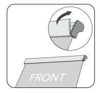
Press down firmly on clamp top bar to secure graphic into place.
