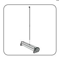
Insert the bottom of the pole in the center of the base.
