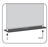
With the frame still laying down, attach the base (D) to the frame with the provided screws (C) and hex key.
