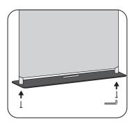
With the frame still laying down, attach the base (D) to the frame with the provided screws (C) and hex key.
