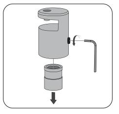
Using a 3mm hex key on the side of the edge grip, loosen the set screw to separate the barrel insert (B) from the cap (A).
