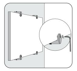
6 Slide in the panel and use a 3mm hex key to tighten the screws on the front of the edge grips - securing the panel in place.
