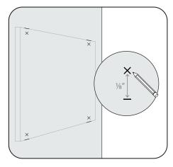
Create new marks 1/8" inset from the original marks made. Drill pilot holes using new marks.
