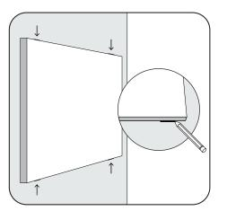
Place panel in desired location and hold steady. Using a pencil, create a mark at the edge of the panel (where it meets the wall) for each edge grip and set panel aside.
