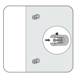
Attach the panel grip to the wall using #6 screw.
