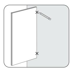
Place panel in desired location and create a mark at the edge of the panel (where it meets the wall) exactly where the panel grips will be installed. Set panel aside.
