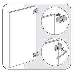
Slide in the panel and tighten using a 2mm hex key.
