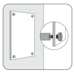
Align the panel. Thread caps (A) through holes in the panel into the barrels (B). To secure into place, handtighten only.
